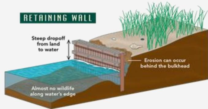
'Hard' infrastructure like retaining walls abruptly severs the ecological connection between the coast and water.
